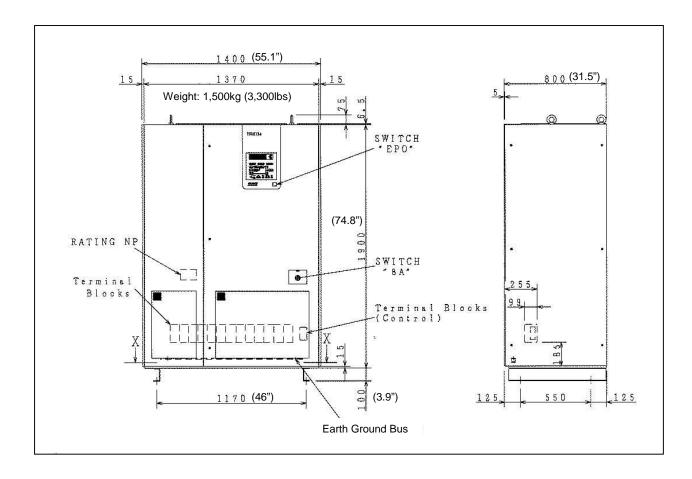
Figure 4 - 150 & 225kVA UPS Exterior dimensions (front & right side).
